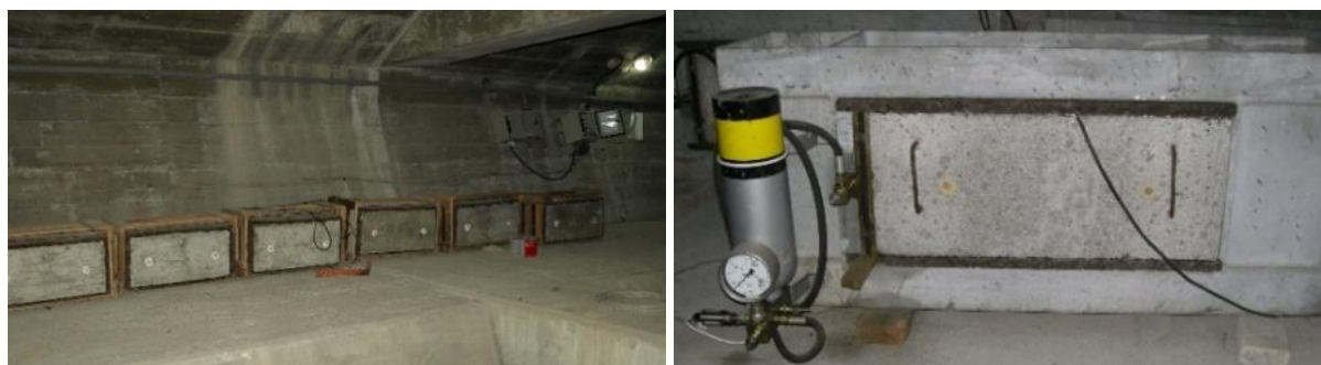
Figure 3. Shrinkage and creep specimens stored inside the deck
