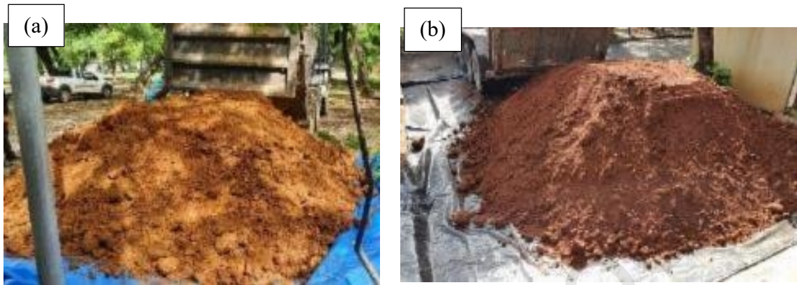
Figure 2. Studied soils: (a) sub-ballast soil; (b) subgrade soil
