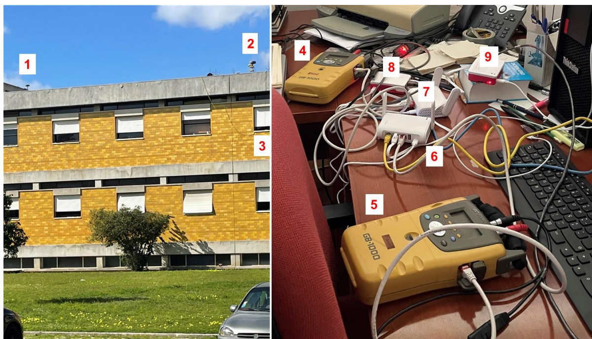
Figura 7.1 – Ensaio com os recetores GNSS Topcon GB-1000: 1 – antena GNSS Topcon choke ring; 2 – antena GNSS Topcon choke ring; 3 – sala onde estavam os recetores GNSS; 4 – recetor GNSS Topcon GB-1000; 5 – recetor GNSS Topcon GB-1000; 6 – modem/router Opal Gi iNet; 7 – modem/router Opal Gi iNet; 8 – Raspberry Pi; e 9 – Raspberry Pi
