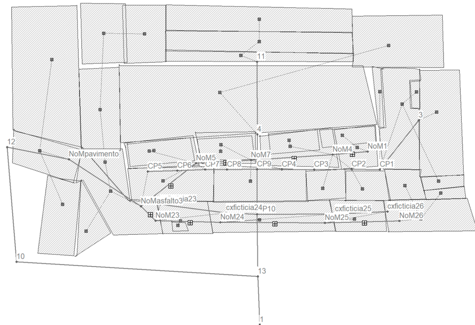
Figure 5. SWMM model schematic representation.
