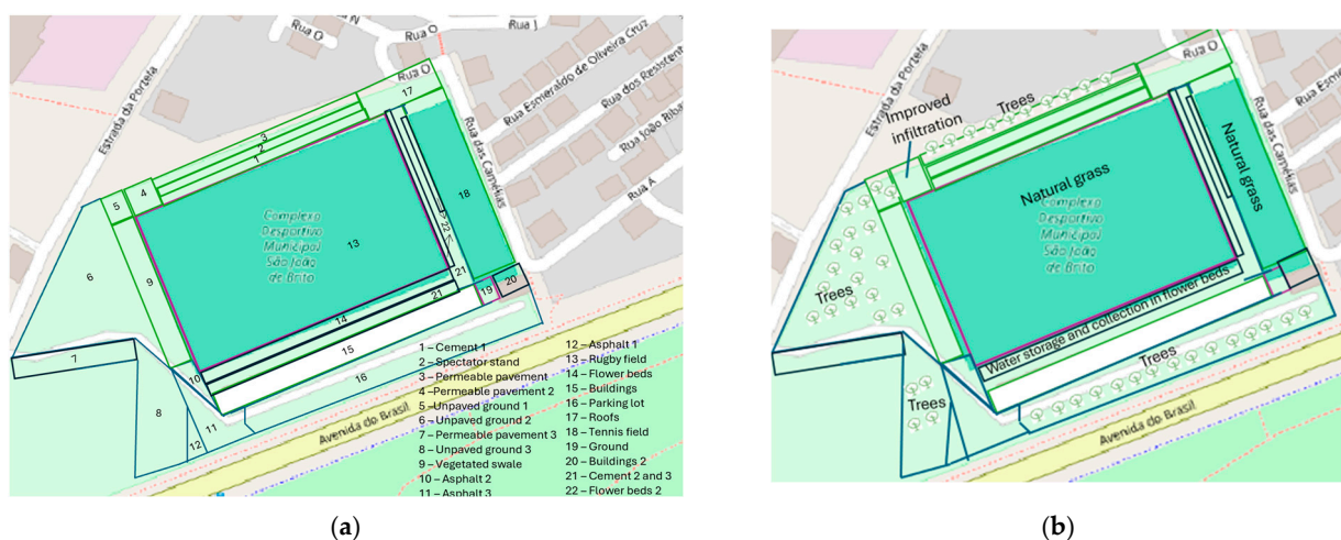
Figure 6. CRSM sub-catchments (a) and planned interventions in Model B (b).
