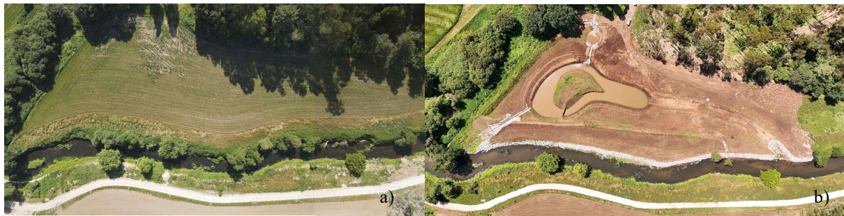
Fig. 1. Retention basin re-naturalized by CRL intervention. a) Before the initial intervention; b) after intervention.
