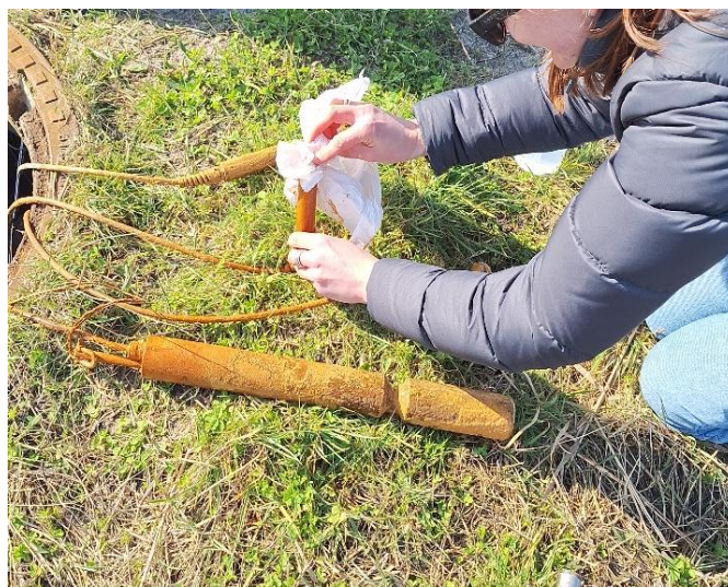
Figure 3.11. Acacia colleagues cleaning the Broekman sensors covered in a red-brown sludge on March 7 th , 2025
