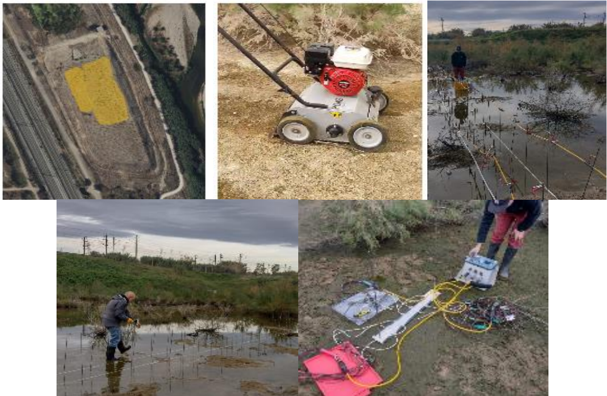
Figure 1.16 Field works: scarified area, scarifying machine and geophysical surveys
