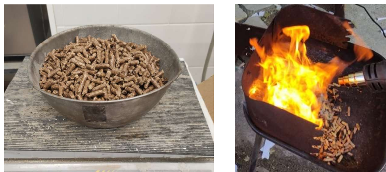
Figure 2. Illustration of firebrand ignition process under simulated wind conditions.
