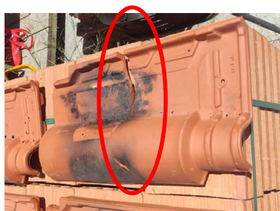
Figure 9. Extreme thermal event of firebrand accumulation that led to severe fracture in the ceramic tile.
