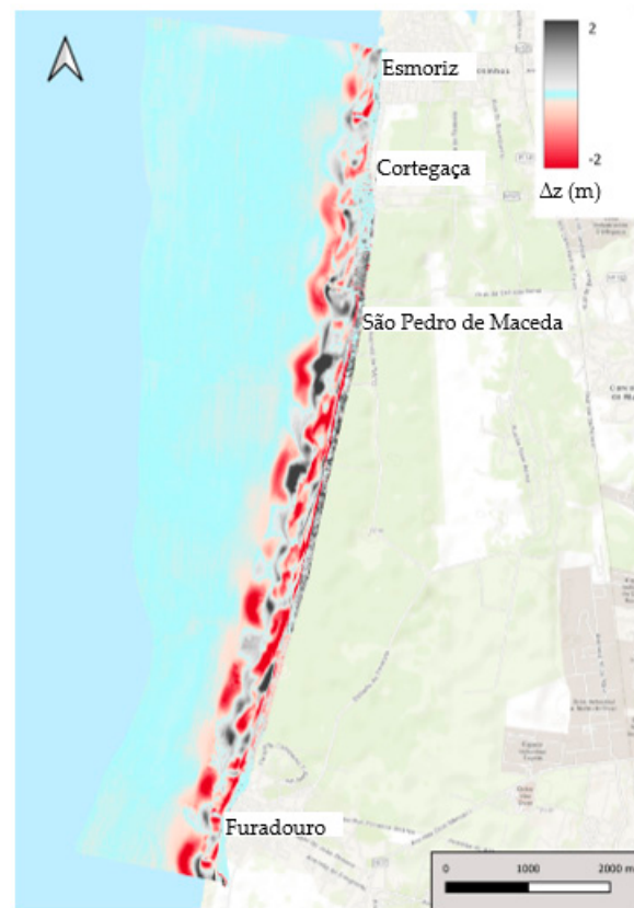
Figure 10. Variation in the vertical level ( \Delta z in m; red corresponds to erosion) between the topobathymetric surveys of September 2018 and July 2020. (Background image: ESRI Topographic basemap. Sources: Esri, HERE, Garmin, Intermap, Increment P Corp., GEBCO, USGS, FAO, NPS, NRCAN, GeoBase, IGN, Kadaster NL, Ordnance Survey, Esri Japan, METI, Esri China (Hong Kong), OpenStreetMap contributors, and the GIS User Community).
