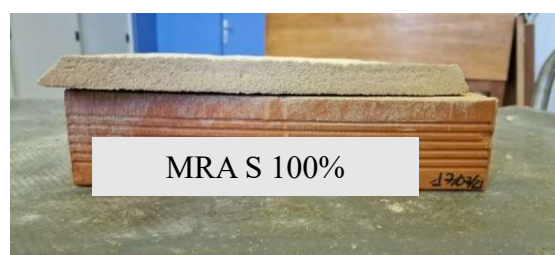
Fig. 4. Lack of adhesion of the mortar MRA S 100%.
