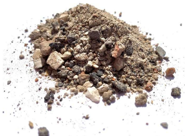
Fig. 1. MRA A as it came from recycling plants (before sieving).
