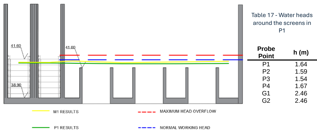
Figure 55 - Comparison of P1 results with experimental results regarding water heads
