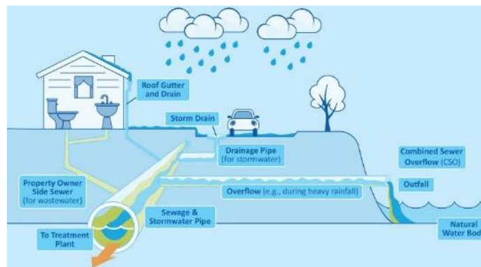
Figure 4 - Combined urban drainage system [15]
