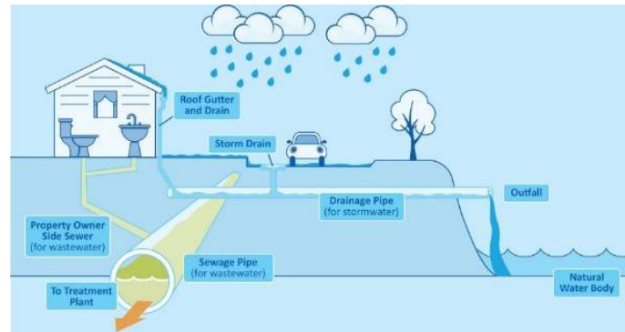
Figure 3 - Separative urban drainage system [14]
