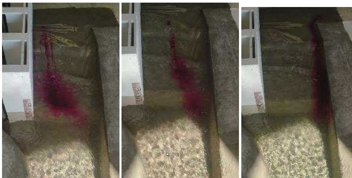
Fig. 19 – Physical model. Level (45.00): Lowered sill and connecting ramp to the secondary channel. Dye plume released upstream of the flow control sill.
