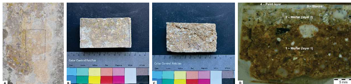
Figure 1. Collection area for one of the samples from the north-facing wall of the staircase (A); external (B) and internal (C) faces of the rendering mortar collected from (A); and stereozoom microscope image of the rendering mortar sample (D)
